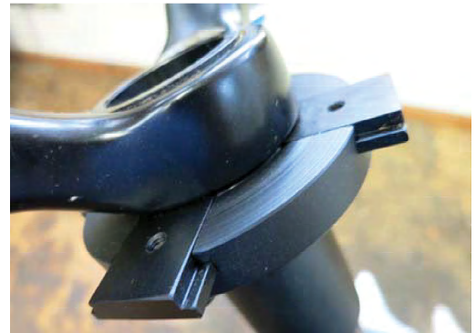
Be sure the jaws stay in place while using the slide hammer to remove the bearing race.
