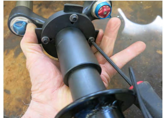
Hold the jaws against the race while tightening the socket head screws.
