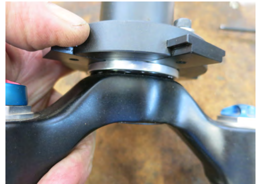
Race installation can be accomplished using the top of the removal tool for 1" and some 1.125" races. A special ring is used for 1.5" races.
