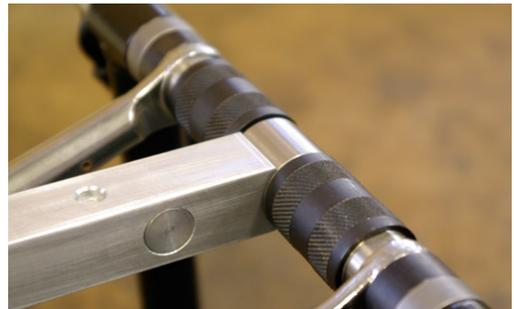
The Target arm may be reversed when using the 40 mm diameter adapters for the dropout alignment tools to obtain greater precision. The 40 mm diameter target is bolted to the end of the target arm in place of the 22 mm target.
